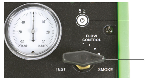
Fig. 9: Smoke flow control fully opened
